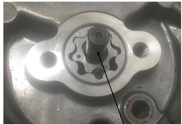
Oil Pump Shaft
