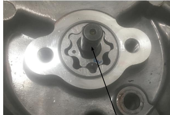
Oil Pump Shaft
