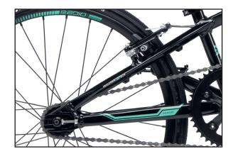
TOP TUBE LENGTH 19.5" HEAD TUBE ANGLE 73.5° BAR RISE 5.75" BACKSWEEP 8° CHAIN STAY LENGTH 13.6" SEAT TUBE ANGLE 71° BAR WIDTH 24.4" UPSWEEP 2°
