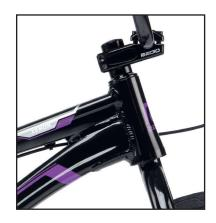
**TOP TUBE LENGTH** 20.75" **HEAD TUBE ANGLE** 74° BAR RISE 7.5" **BACKSWEEP** 11° 3.5° **CHAIN STAY LENGTH** 14.25" **SEAT TUBE ANGLE** 71° **BAR WIDTH** 28" **UPSWEEP**
