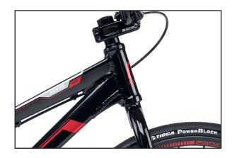
TOP TUBE LENGTH 17.6" HEAD TUBE ANGLE 73° BAR RISE 2.25" BACKSWEEP 8°
