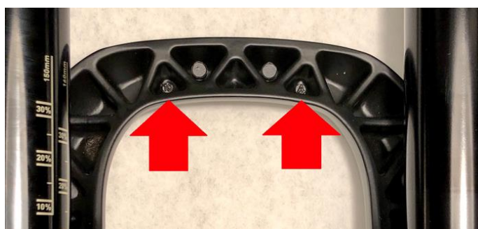
Casting code on the inside of arch web:
